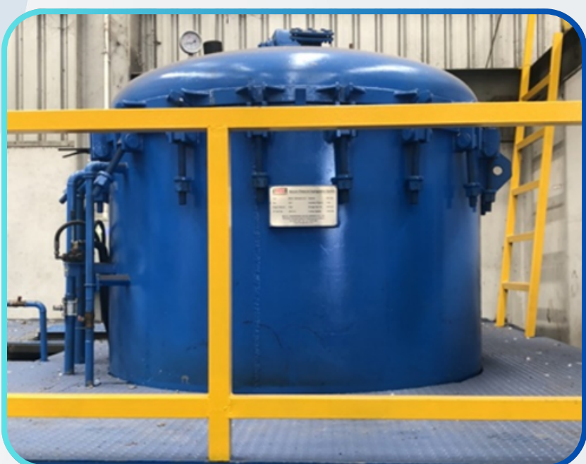
Vacuum Pressure Impregnation Diameter 1.5x2.5 Meter
