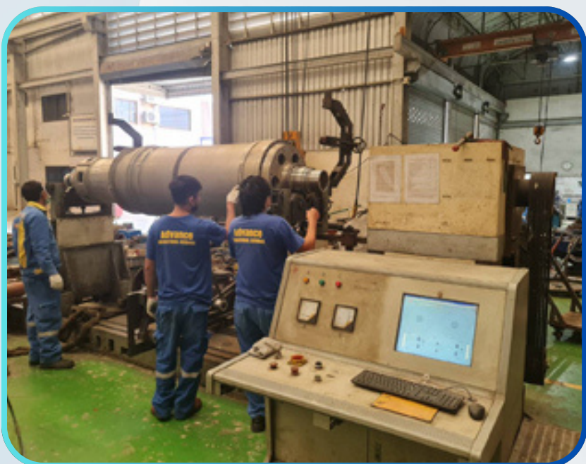
Balancing machines 3 Unit 10 Tons 4 Tons 100 Kg.
